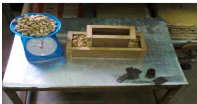
Fig. 6 Determination of coefficient of static friction
