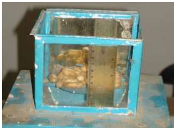
Fig. 5 Determination of angle of repose
