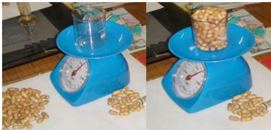
Fig. 3 Measurement of bulk density
