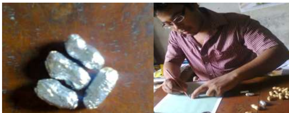
Fig. 2 Surface area determination by surface coating method
