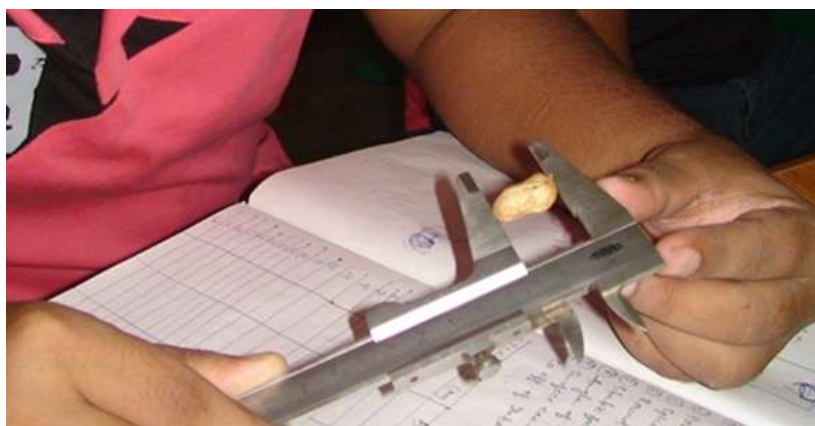
Fig.1 Measurement of length, width and thickness of groundnut
