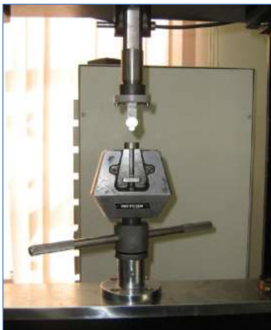
Fig-4: Universal testing machine (instron) with 5 mm diameter stainless steel ball using for applying load on the alumina cores
