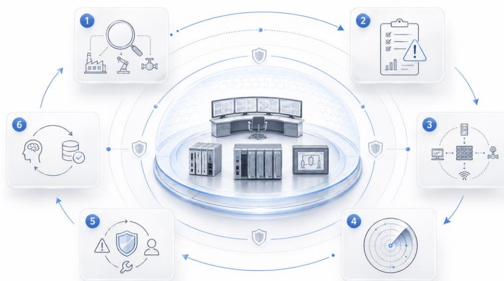
Figure 2: Cyber resilience lifecycle for industrial control systems: asset discovery, risk assessment, segmentation, continuous monitoring, incident response, recovery, and continuous improvement.
