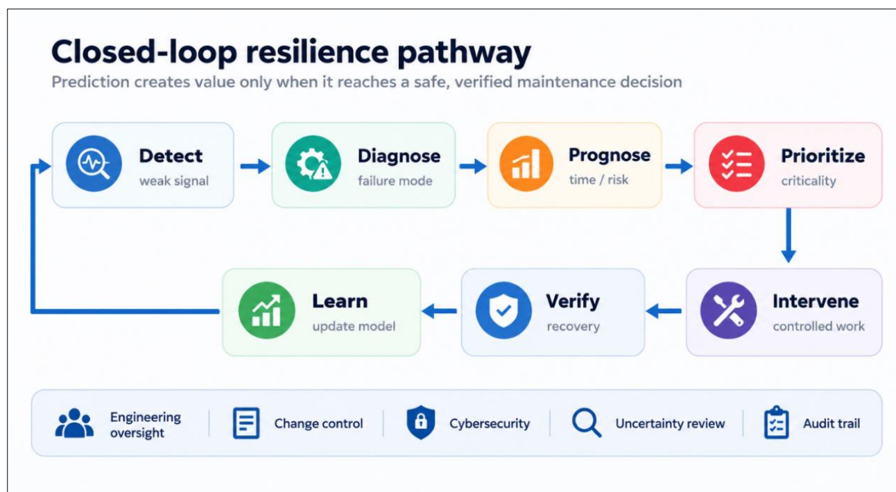
Figure 2: Closed-loop pathway through which predictive maintenance contributes to resilience, with engineering oversight and governance spanning the full cycle
